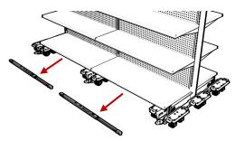
Mobilize fixture using pull bar inserted into pull hooks on skate.
